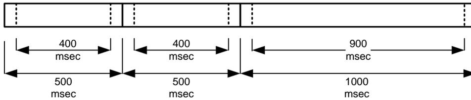
Figure 4-2 Example of slot occupancy
