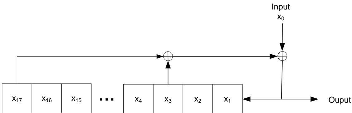
Preload shift register with 0x01 prior to start
