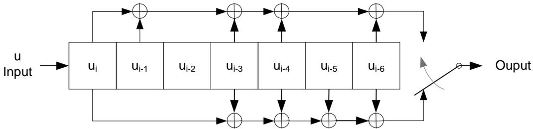
Figure 3-5 Block Diagram of Rate  $1/2$   $k=7$  Convolutional Encoder
